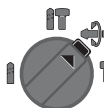
Vario-Lock position for adjustment of the chiselling position. The mode selector switch does not latch in this position.
